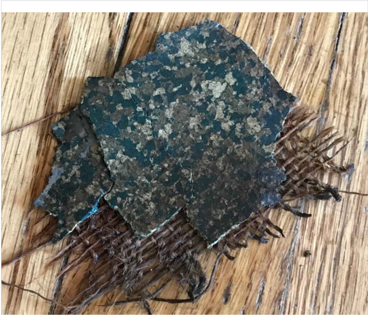
ADDITION ROOM 5 - SAMPLE FROM FIRST LAYER OF LINOLEUM, BEE LAB PHOTO Note: The colors of this sample are inherent from surface to base, and have been melted together to form the sheet.
